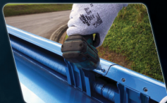
Air conditioning piping is routed on the outside of the vehicle, a system that facilitates maintenance.
