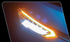
Full LED improved light set with long-range lights and maneuvering light.
