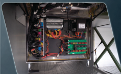
Optimized wiring harness routing, making maintenance and distribution of electronic components easier.
