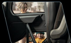
Translucent area on the door allows obstacles on the side of the vehicle to be seen.
